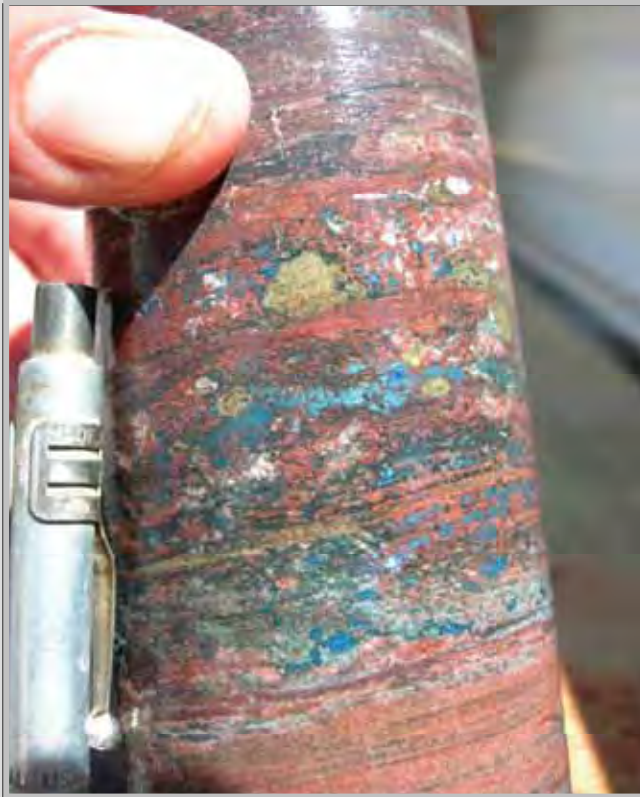
Examples of copper sulphide mineralisation in the Groundhog hole (GHDD1)
