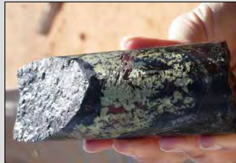
Chalcopryite in chlorite-hematite alteration
