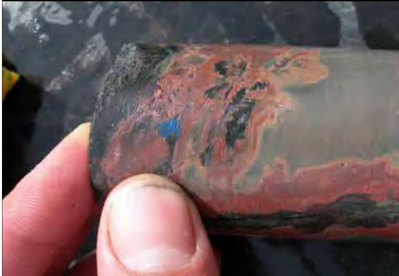
Bornite in hematite-albite-chlorite altered volcanics
