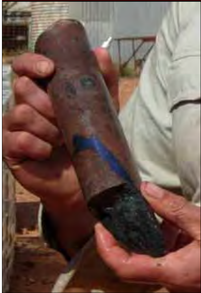
Bornite in hematite altered volcanics
