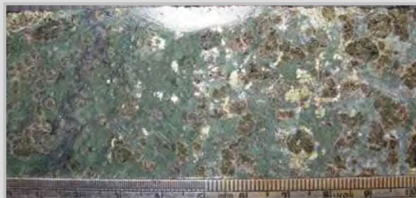
chlorite/carbonate (siderite) alteration with chalcopyrite and pyrite
