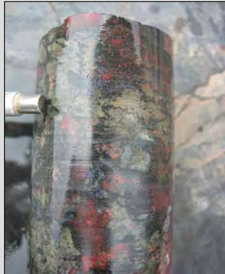
Bornite in amphibole-chlorite-hematite altered volcanics
