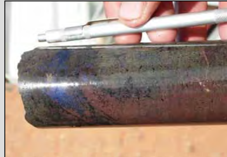
Bornite and minor chalcopryite in hematite-amphibole-chlorite alteration
