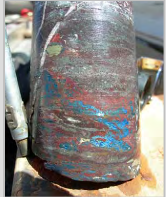
Examples of copper sulphide mineralisation in the Groundhog hole (GHDD1)
