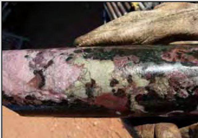
Chalcopryite in chlorite-hematite- carbonate alteration
