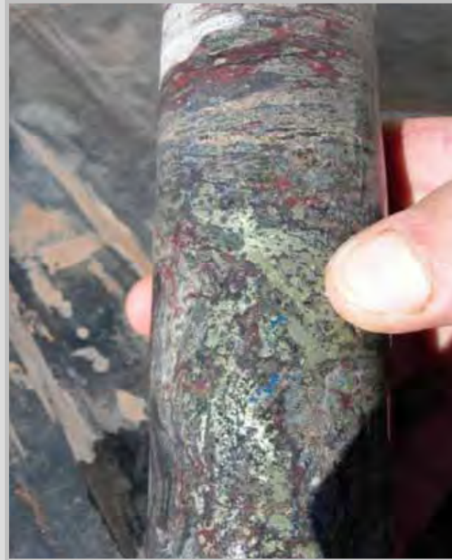
Examples of copper sulphide mineralisation in the Groundhog hole (GHDD1)
