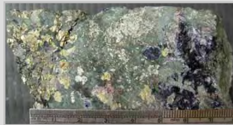
amphibole/chlorite alteration with chalcopyrite, pyrite and fluorite
