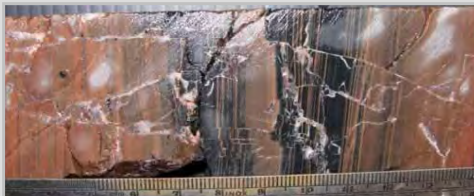
hematite altered mudstone/siltstone with carbonate veining
