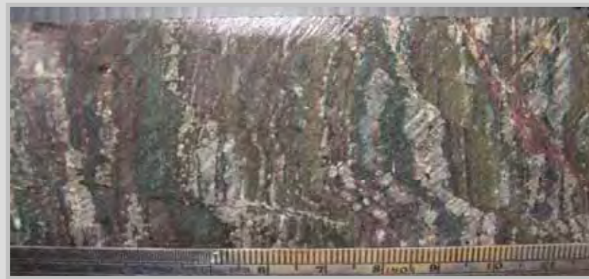
intense amphibole/chlorite/carbonate alteration overprinting hematite/albite alteration
